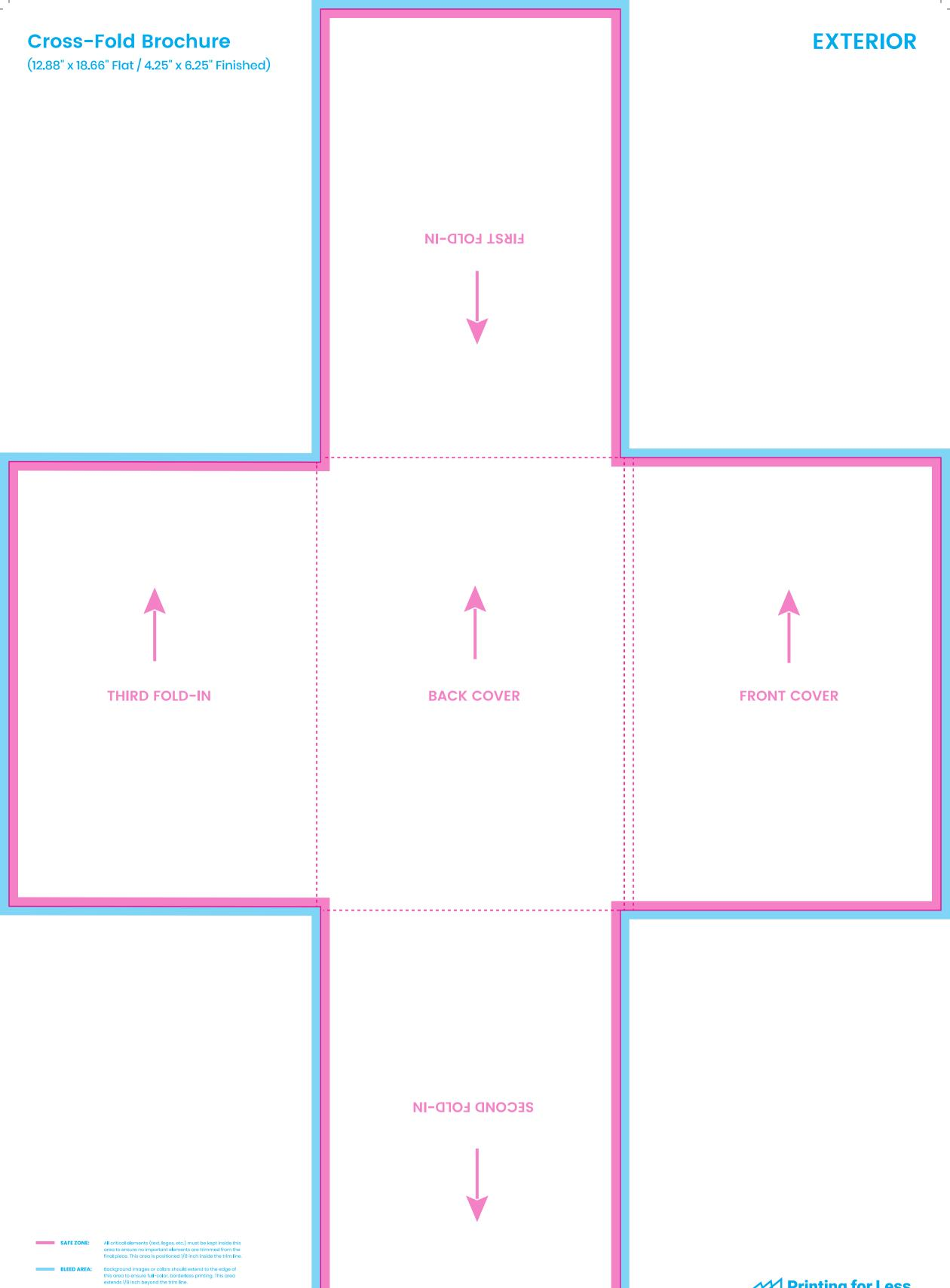
The trim line represents where the piece will be cut and indicates the final size of the piece. Pro Tip: Due to production variance, it's recommended to keep borders at least 1/8 inch away from the trim line or avoid them completely.
